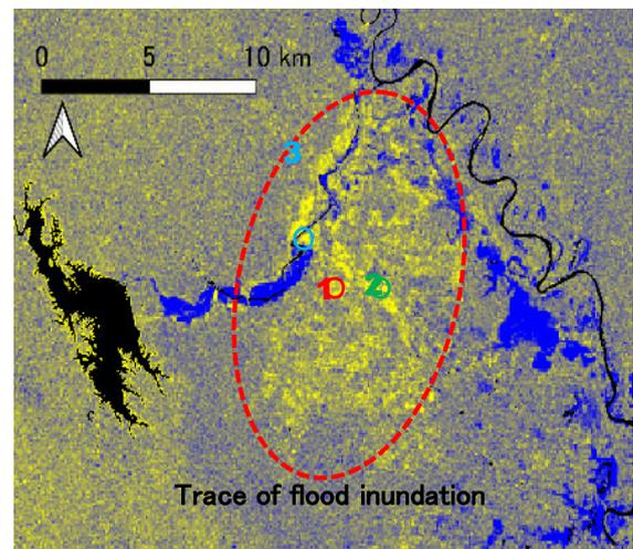
Change in VH polarization from Sentinel-1 SAR images before and after the flood. Yellow indicates an increase, and blue indicates a decrease. Black is the water surface before the flood. The yellow area is assumed to be a trace of the flood inundation area because it is thought to capture changes in surface conditions such as rice being pushed over by turbid water.
