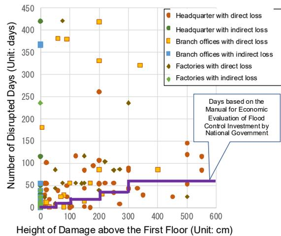
Relationship between the floodwater level above first floor and the days of business suspension due to the July 2018 heavy rain
