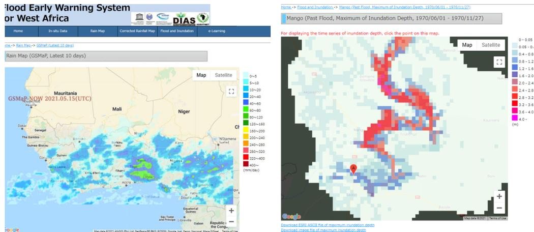
GSMaP real-time visualization (left) and expected maximum inundation depths at hot spots (right) on the FEWS
