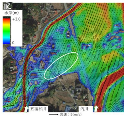
The results of flood flow computation in the Gofukuya River (The color counters show flow depths at the peak discharge.)
