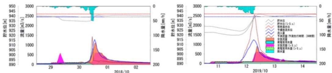
Results of dam operation during the flood caused by a typhoon at Hatanagi Daiiti Dam
