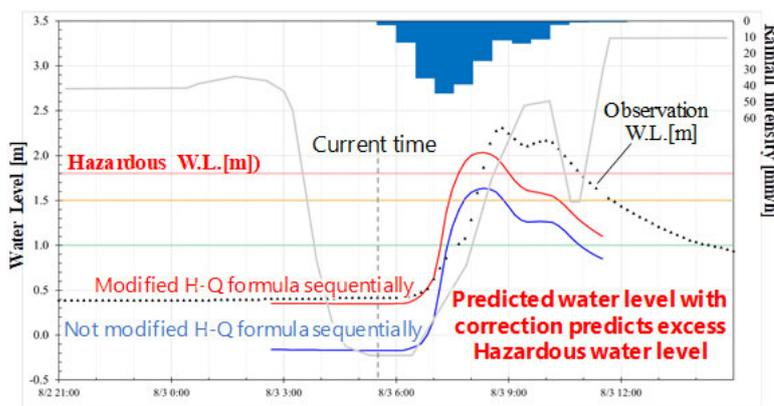
Comparison example of predicted water level with and without H-Q curve sequential correction
