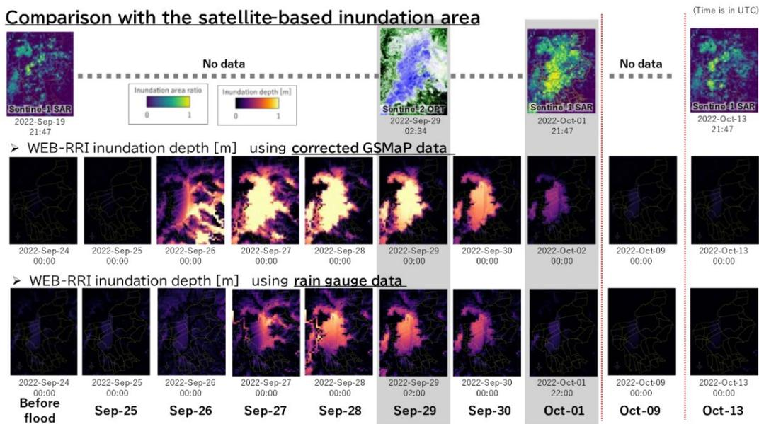
Fig. 3-2 Comparison between satellite-based and RRI-based inundation extent in Kandaba City, the Philippines
