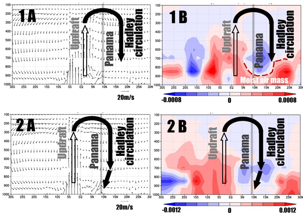
Fig. 3-5 The north-south vertical cross-sections, created using the DIAS vertical cross-section analysis tool, exhibiting the difference in vertical wind speed (A) and specific humidity in the atmosphere between their 20-year average and the wet-year average (1A&B) and the drought year (2A&B)
