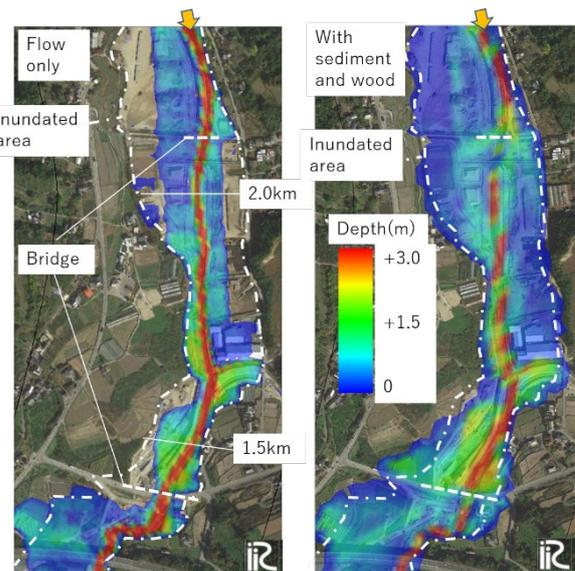
Fig. 3-7 A comparison in the water depth the peak discharge between water only (left) and water with sediment and driftwood (right) (The white dotted line indicates the flooded area interpreted from aerial photos)
