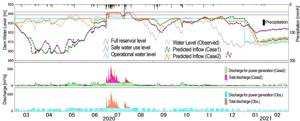
Fig. 3-10 The simulation results of the annual operation of the Oi Hatanagi 1 Dam for the period of March 2020 - February 2021
