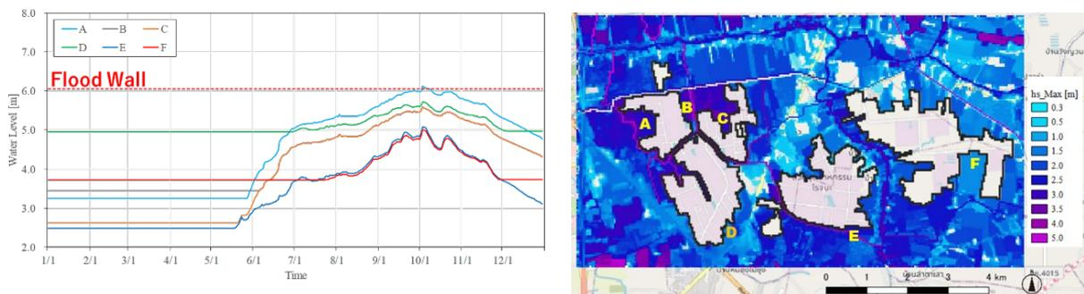
Fig. 3-9 Inundation depths at six locations when a rainfall event of the historical maximum scale occurs over the basin every month
