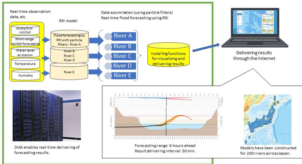
Fig. 2-2 Outline of flood forecasting system for small and medium rivers
