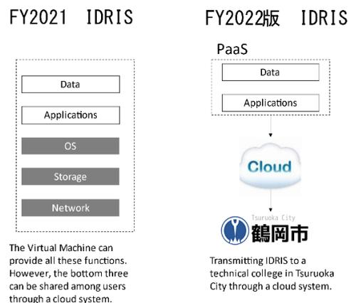
Fig. 3-12 Comparison of two versions of IDRIS
