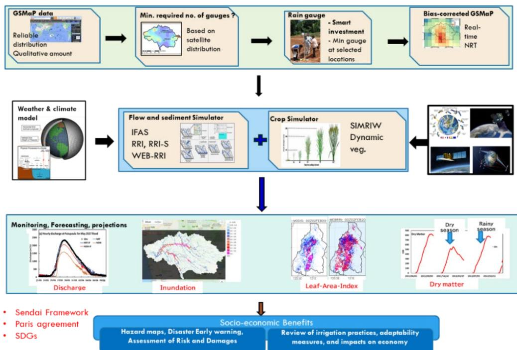
Fig. 3-1 A system for the integrated management of water resources and disasters in poorly gauged basins
