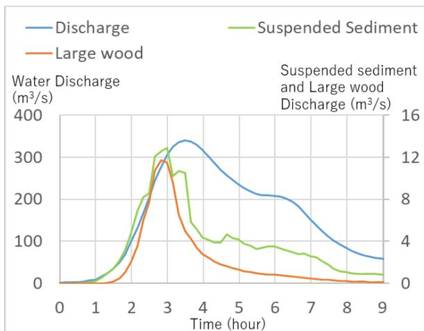
Fig. 3-6 The estimated discharges of water, sediment, and driftwood in the 2017 Akatani River flood
