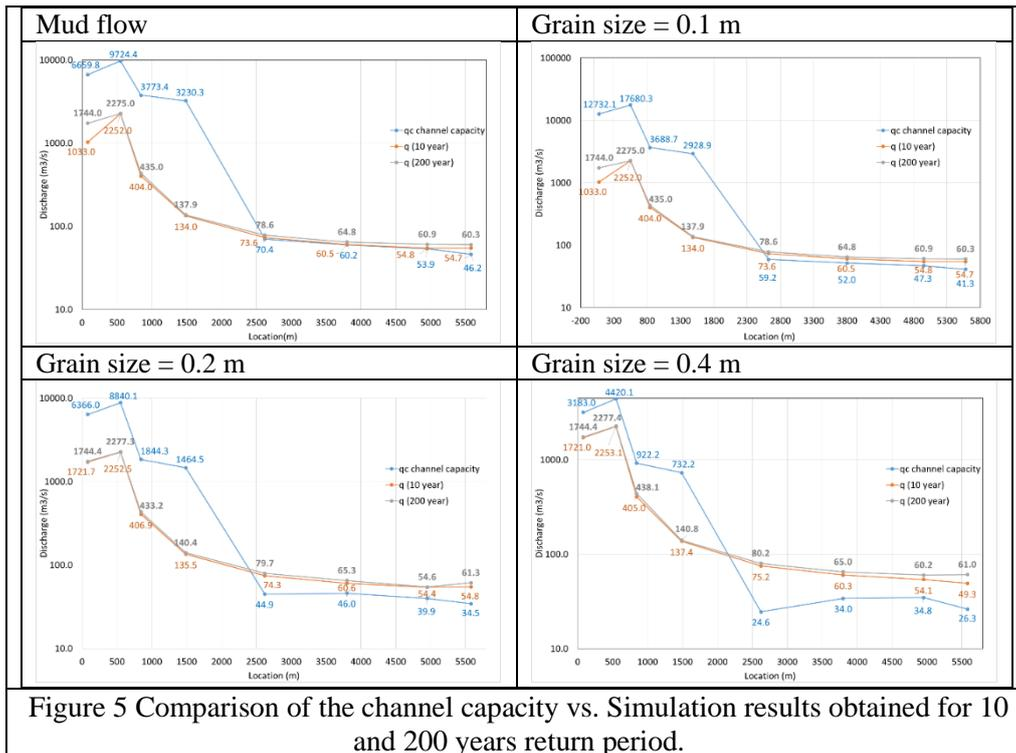
Figure 5 Comparison of the channel capacity vs. Simulation results obtained for 10 and 200 years return period.
