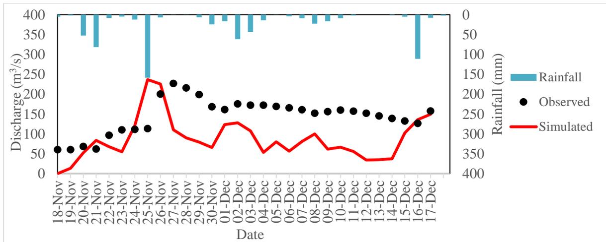
Figure 3: Observed and simulated hydrograph at Nabua station for November 18 to December 17, 1987.
