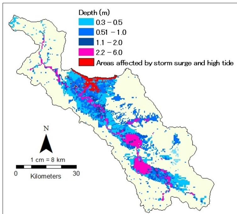
Figure 6: Composite Map from hydro-geomorphic method and hydrologic modelling method with design rainfall of 100 year return period.
