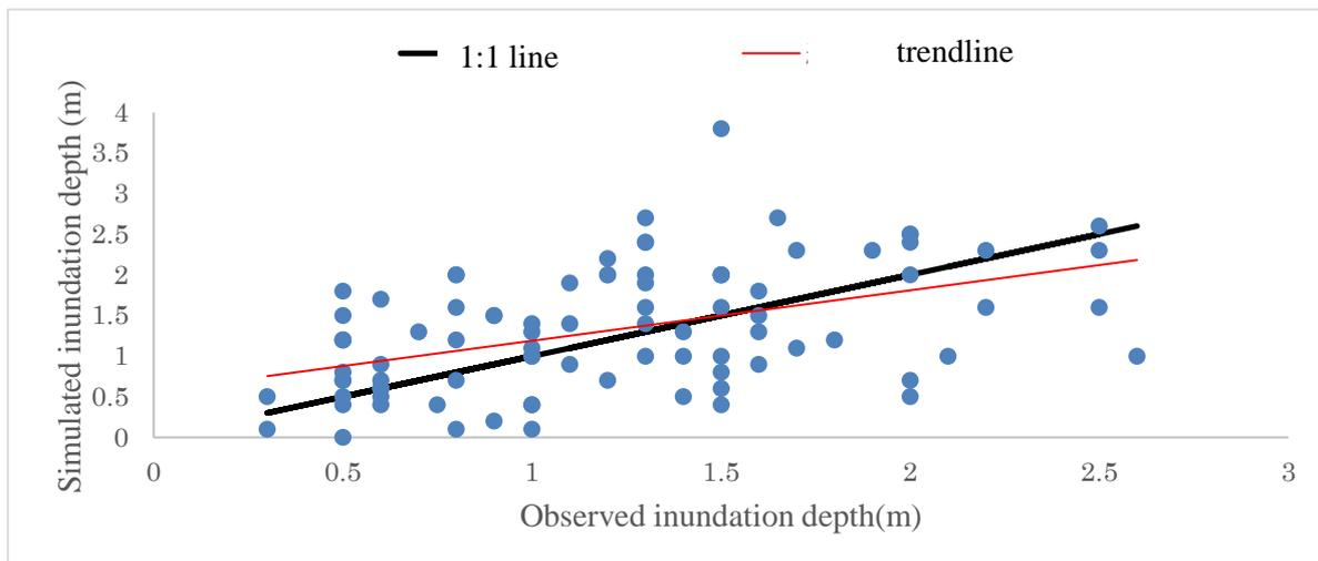
Figure 4: Scatter plot diagram of the observed and expected inundation depths of the 1995 flood event simulation.
