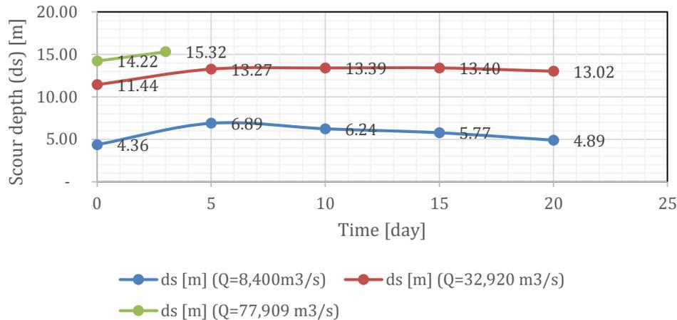
**Figure 5.4 Variation in time of the local scour depth at bridge pier**
