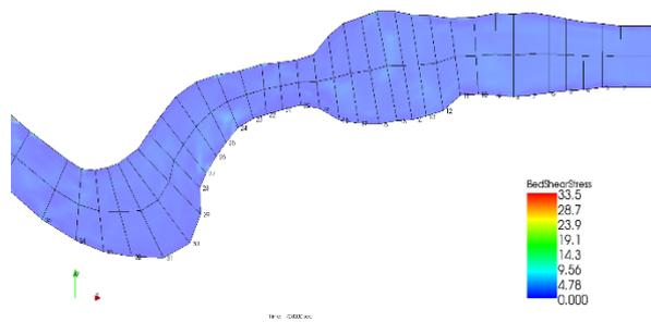
**Figure 5.1 Bed shear stress of the Study Area for 20days computation**
