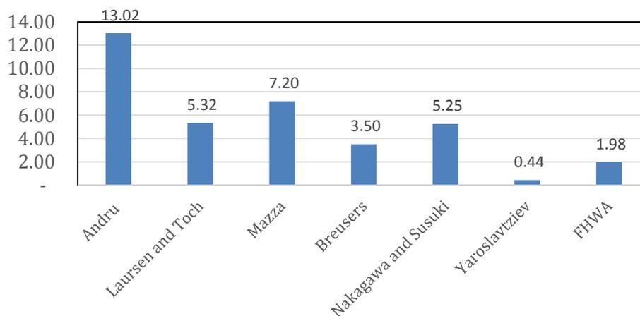
**Figure 5.3 Maximum possible local scour depth at piers in meters**
