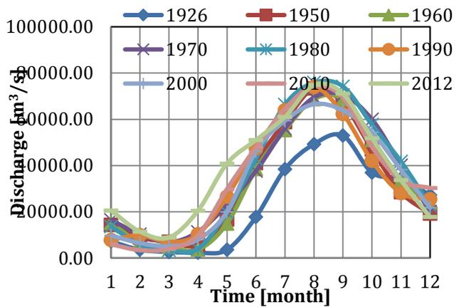
Figure 3.3 Monthly discharge of Orinoco River at Caicara Gauge Station Jan -1926 to Dec -2012
