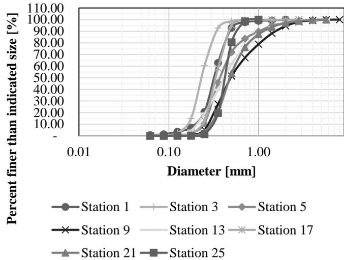
Figure 3.4 Particle size distribution of bed material Orinoco River
