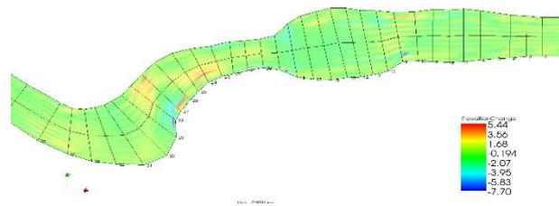
**Figure 5.2 Elevation change of the Study Area for 20days computation**
