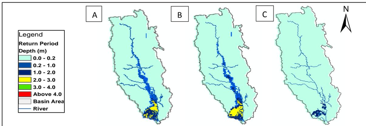
Figure 6. The spatial distribution of flood extend area by different countermeasures for 3m high embankment construction(A), dam constructions(B) and combination of embankment with dam constructions(C).
