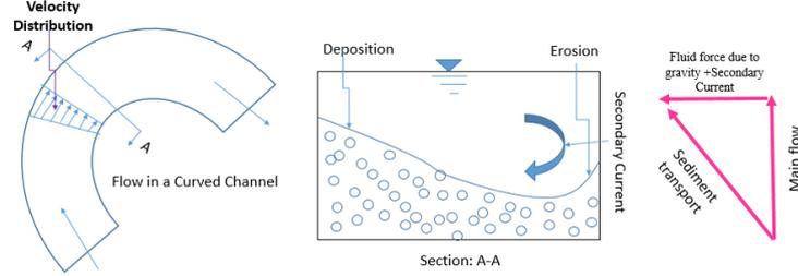
Figure 2. Flow in a curved channel
