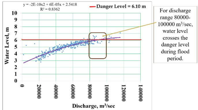
Figure 4. Stage-discharge relationship of Padma River at Mawa point (Source : FFWC, BWDB)
