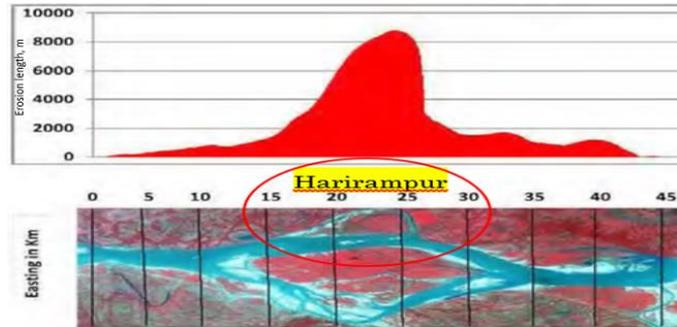
Figure 5. Bank erosion pattern along the left bank of Padma river at Harirampur area (nhc., 2013)
