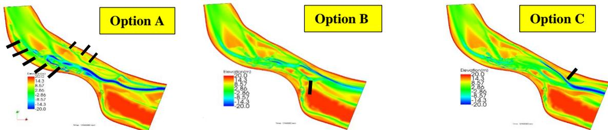
Figure 5: One flood (150 days) simulation result with spur dike location (//)
