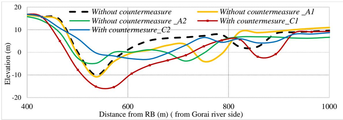
**Figure 8: Cross-section comparison near the Gorai off-take**
