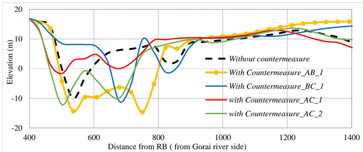
**Figure 10: Cross-section comparison near the Gorai off-take**
