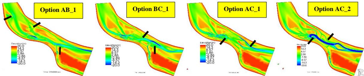
**Figure 9: One flood (150 days) simulation result with spur dike location ( // )**
