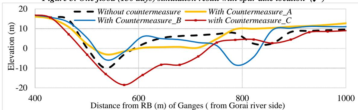
Figure 6: Cross-section comparison near the Gorai off-take
