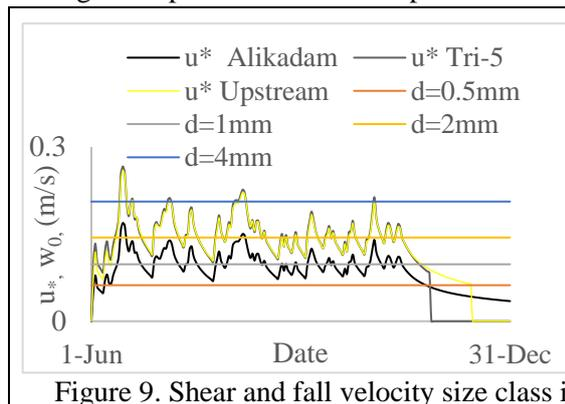
Figure 9. Shear and fall velocity size class i
