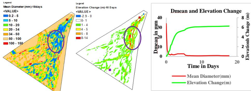
Figure 5: Comparison of sediment diameter and elevation change.
