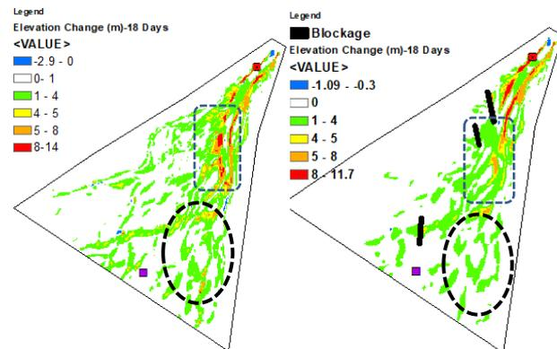
Figure 9: Comparison of sediment deposition height with and without countermeasures.
