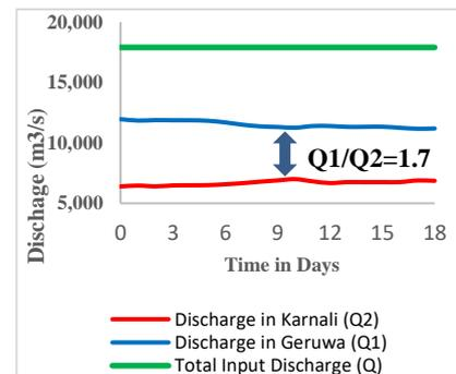
**Figure 11: Discharge distribution among two branches with countermeasures.**
