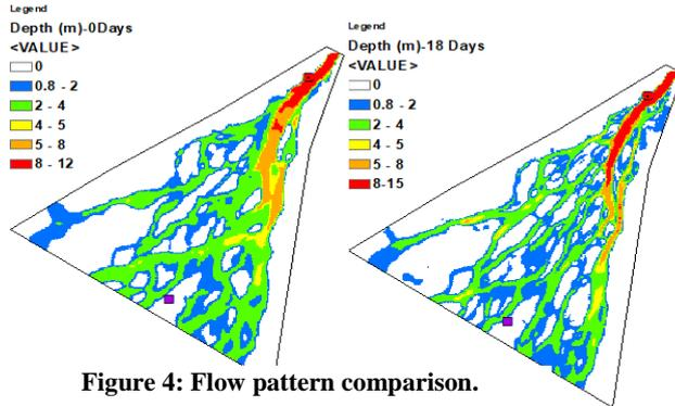
**Figure 4: Flow pattern comparison.**
