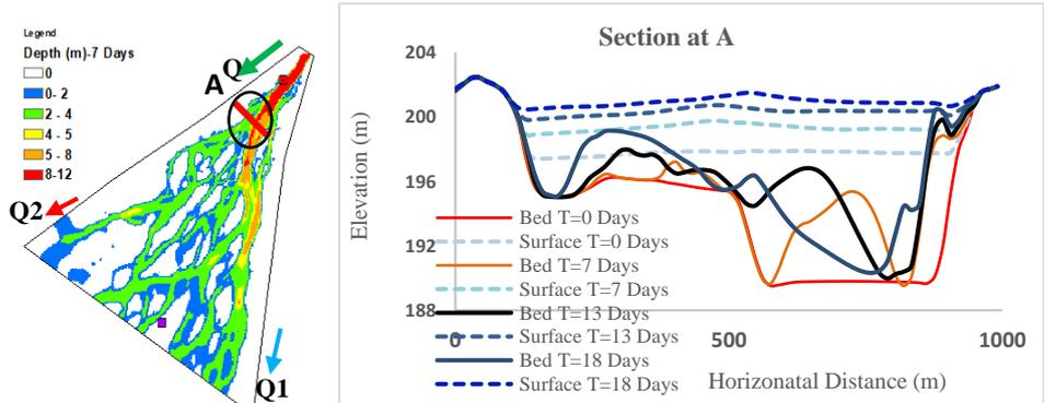
Figure 6: Temporal change in bed elevation at point A.
