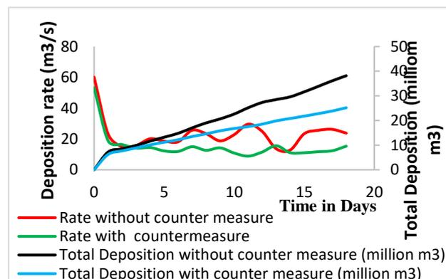
Figure 10: Suspended sediment deposition with and without countermeasures.
