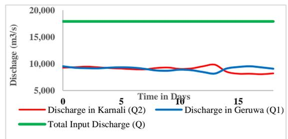
Figure 7: Discharge distribution in two branches
