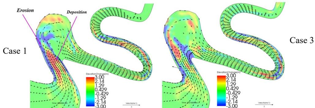
Figure 9. Comparison of bed deformation profile between Case 1 and Case 3 after 30 days of numerical computation
