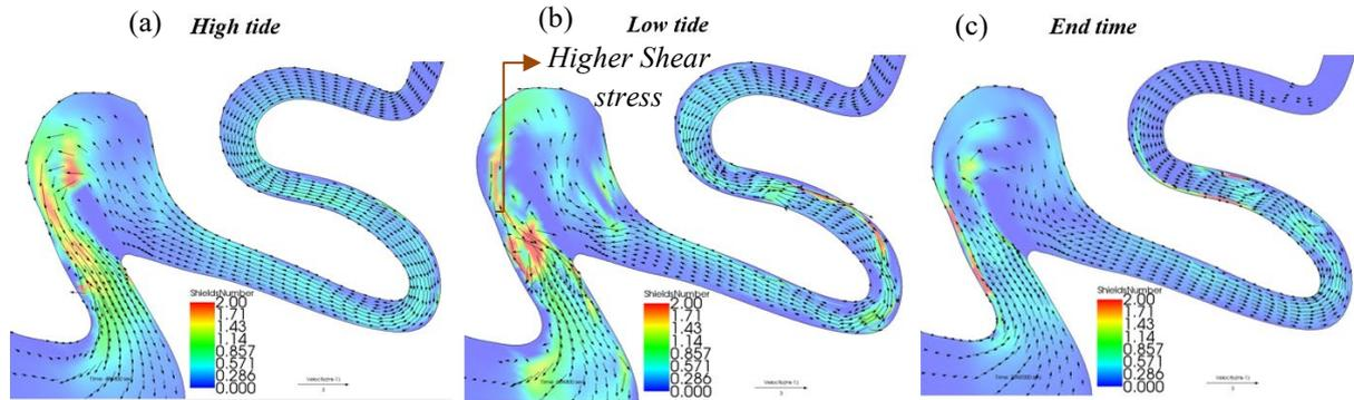
Figure 5. Shear stress profile in Case 1 (a) during high tide, (b) during low tide and (c) at end of computation.
