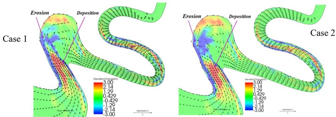
Figure 8. Comparison of shear stress profile between Case 1 and Case 2 during low tide riverbank
