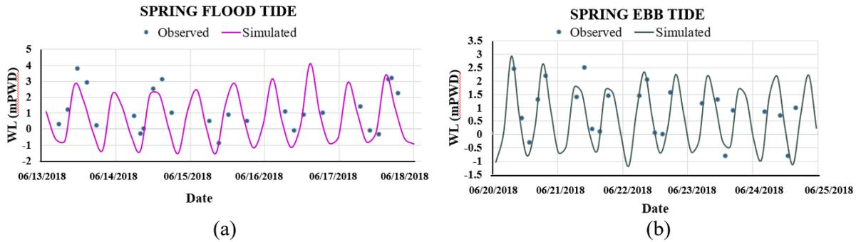
Figure 4. Comparison of simulated water level with observed tidal water level (a) for a spring tide and (b) for a neap tide at station nearby downstream.
