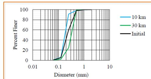
Figure 3. Initial size distribution of sediment particle of bed materials
