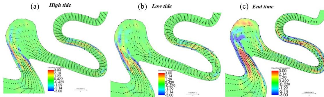
Figure 6. Bed deformation profile in Case 1 (a) during high tide, (b) during low tide and (c) at end of (after 30 days) computation.
