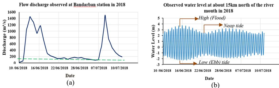
Figure 2. Flow discharge observed at Bandarban station in 2018 and (b) Observed water level at about 15Km north of river mouth in 2018.
