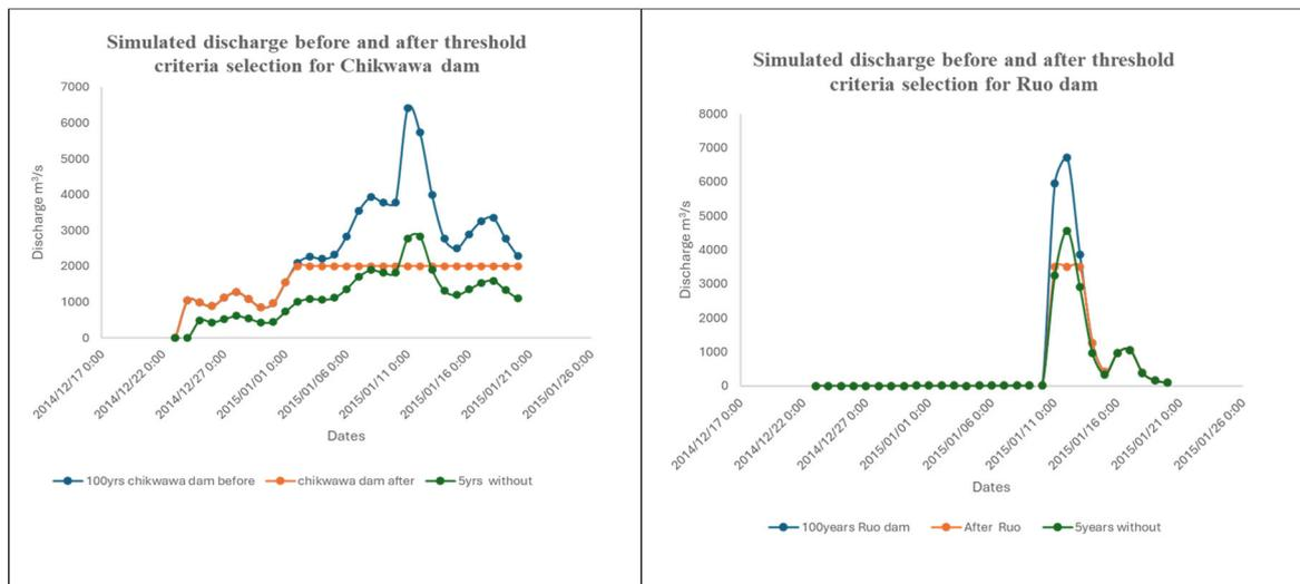
Figure 6: Simulated discharge before and after threshold criteria selection for Chikwawa and Ruo dams
