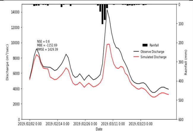
Figure 4: Comparison of calculated and observed discharge for 2018-2019 flooding event
