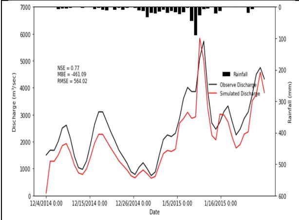
Figure 3: Comparison of calculated and observed discharge for 2014-2015 flooding
