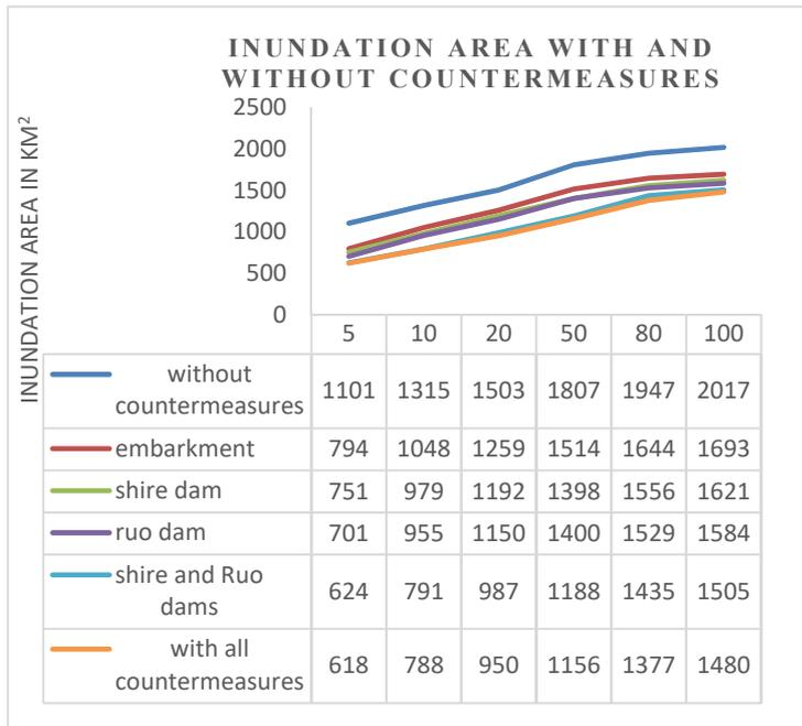
Figure 5: Affected inundation area with and without countermeasures
