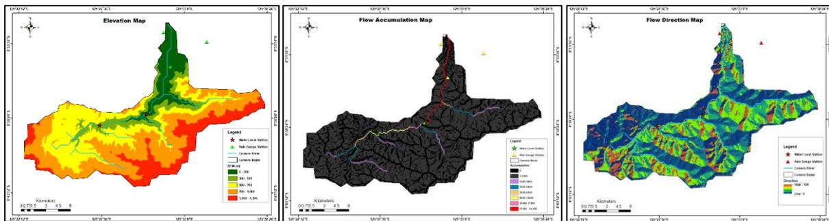
Figure 3. Topography input data: a). DEM, b). ACC, c). DIR for simulation by RRI model.
