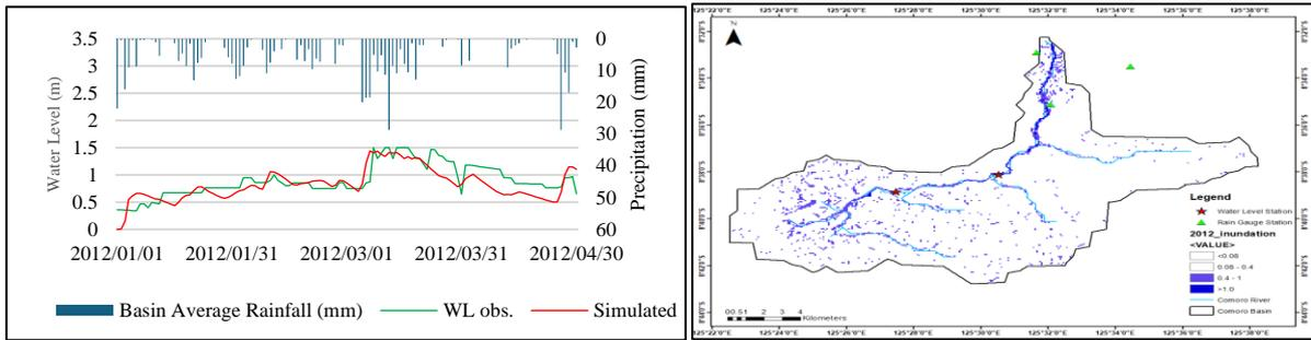
Figure.4. Calibration of RRI model for flood events from January to April 2012.
