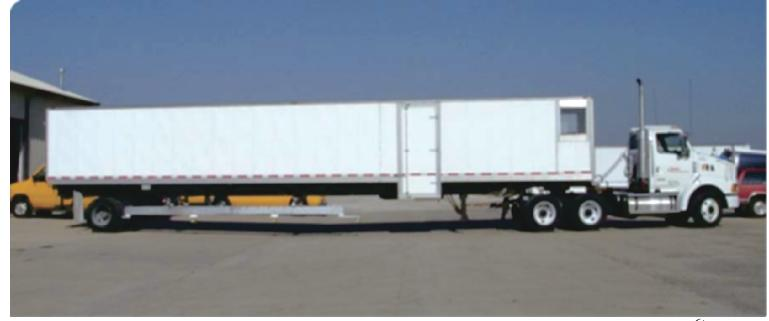
写真-2 RWD (Rolling Wheel Deflectometer (米国))<sup>6)</sup>
