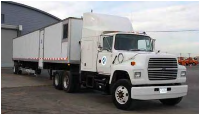
RWD 1) (Rolling Wheel Deflectometer, 米国)
