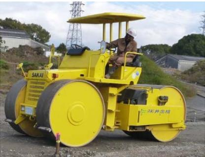
A photograph of a yellow Sakai macadam roller. The machine is viewed from a side-rear angle, showing its two large, heavy-duty rollers. The operator's seat and canopy are visible. The brand name 'SAKAI' is printed on the side of the front roller. The machine is situated on a gravel or macadam surface, with a utility pole and some buildings in the background under a clear sky. |
