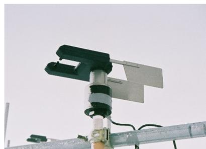
図9 Snow Particle Counter (SPC) の外観
