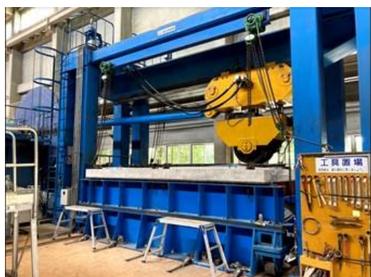
Figure 3: Wheel running machine
