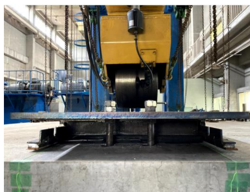
Figure 3: Wheel running machine
