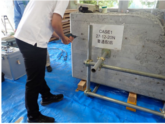
Photograph 7: Experience with a non-destructive testing method (rebound hammer).
