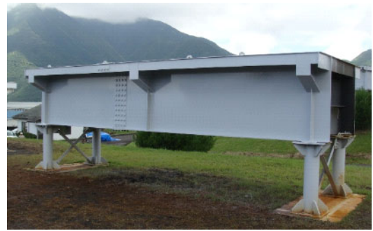
Photograph 2: Large-scale test specimen simulating an actual bridge structure.
