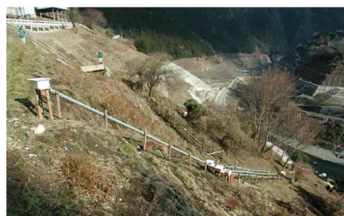
▲伸縮計による移動状況調査 Measurement of ground displacement by using an extensometer
